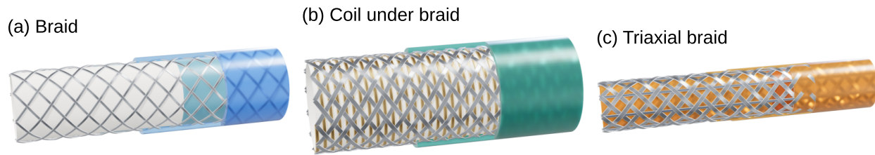
Figure 1. Three shaft construction examples, shown with the wire geometry of the FEM model. The outer polymer layers are cut back. (a) Braid of 16 ribbon wires over a liner. (b) Ribbon coil under a 24-wire braid. (c) Triaxial braid: a braid with straight axial wires. The colours of the polymer layers are for legibility only.
